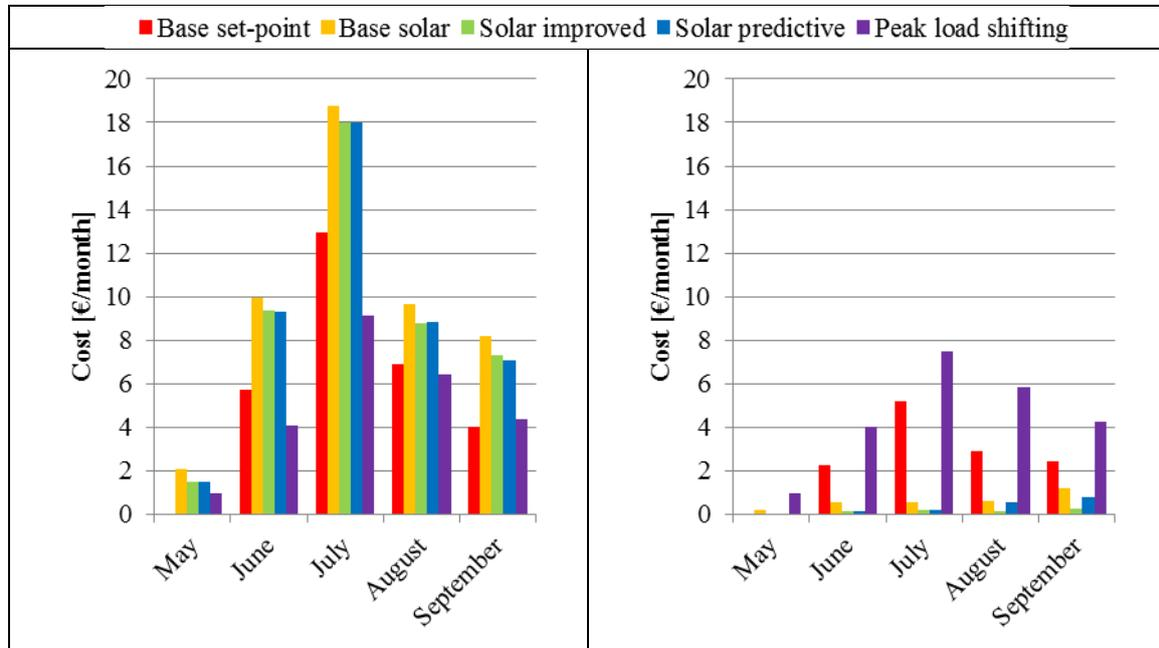
Figure 2. Operation cost without self-consumption (left) and with self-consumption (right) for all control strategies
