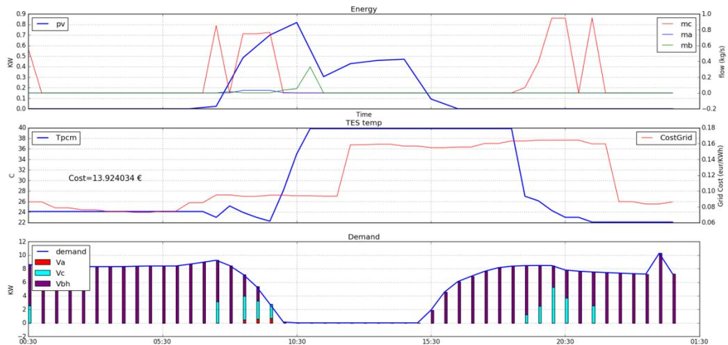
**Figure 2:** The one-day simulation with MPC method
