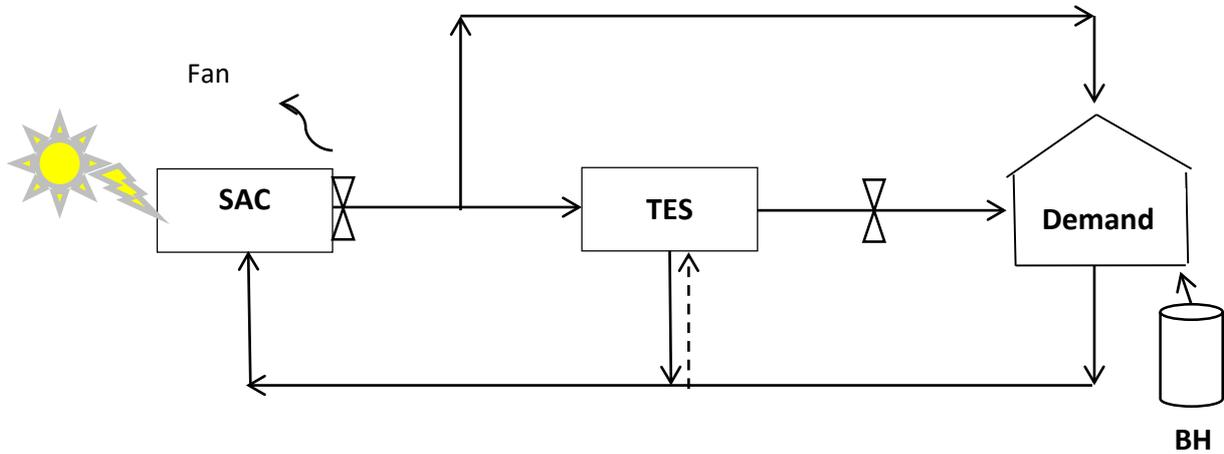
**Figure 1:** Operation scheme of the system
