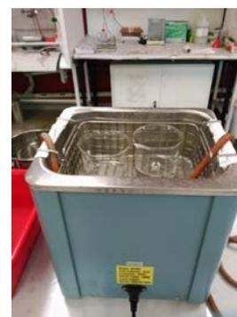
Figure 2. Pictures of the ultrasonic bath and samples when synthesizing nanoparticles and the nanofluid at the lab
