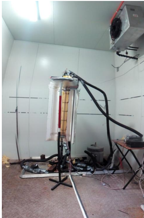
Fig. 1. Shell-and-tube heat exchanger used in the present experimentation.
