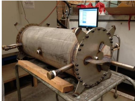
**Figure 1.** A laboratory scale prototype shell-and-tube phase change thermal storage system.
