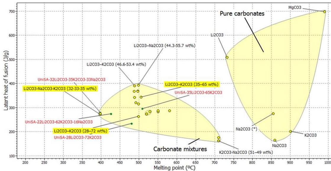
Figure 3.- Thermal properties of different carbonate mixtures, including those used for corrosion experiments during this secondment (UniSA labeled).
