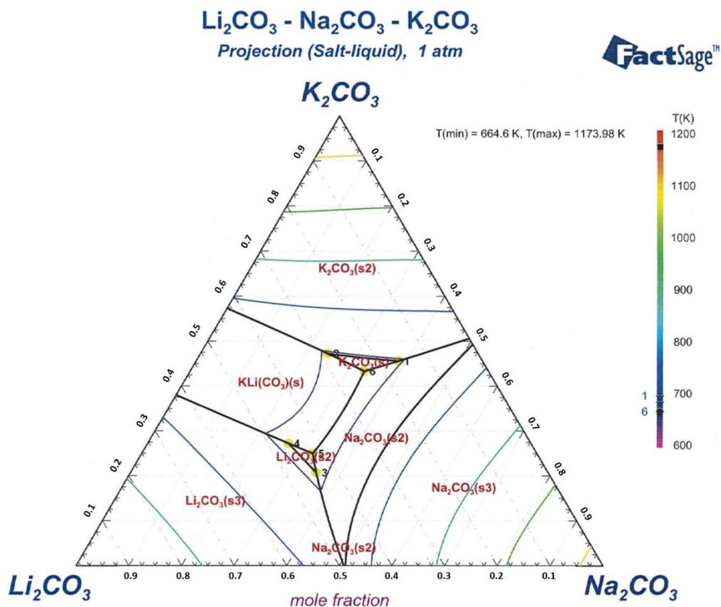
**Figure 1.-** Phase diagram salt-liquid projection, obtained with **FactSage**® - Phase Diagram module, for the Li<sub>2</sub>CO<sub>3</sub>-Na<sub>2</sub>CO<sub>3</sub>-K<sub>2</sub>CO<sub>3</sub> system at atmospheric pressure.
