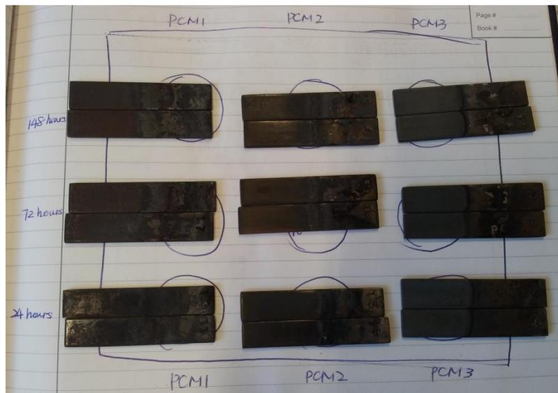
**Figure 2.-** Samples of 316 SS after being immersed in the carbonate salt mixtures at 580°C for different times.
