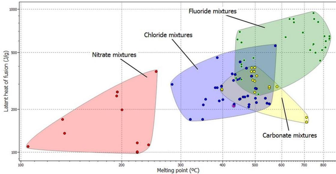
Figure 2.- Thermal properties of different salts.
