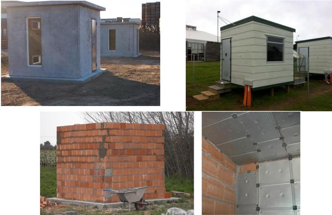
Figure 2 Experimental set-up used for the evaluation. Top left: concrete cubicle; top right: timber hut; bottom: alveolar brick cubicle.
